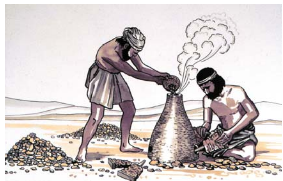
Metallurgy in Arabia. Fig. 9 Based on many fragments a pear-shaped smelting furnace could be reconstructed for the third millennium BCE. But in contrast to this artist's view the bellows most probably were simple skin bellows.
